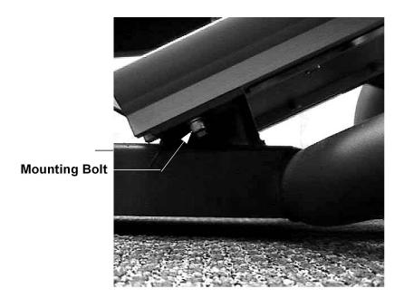
5. Remove the two mounting bolts from the front bottom of the ramp assembly. These bolts fasten the ramp to its front support.
